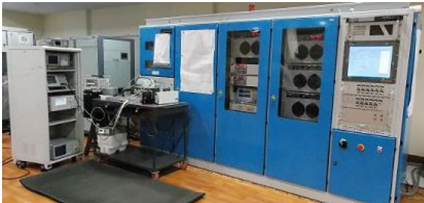
Fig 3. Testing of TWT with Hazemeyer power supply
